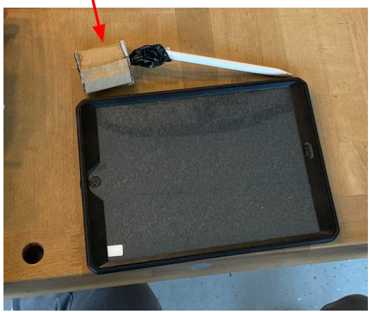
Retractable wire inside cardboard box attached to end of pen
